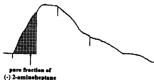
Fig. 3. Elution profile of the so-called "intermediate" and GC analysis of the hatched fraction. Conditions: sample, 2.3 mg of ( \pm )-2-aminoheptane; mobile phase, 0.1 M ( - )- \alpha -methylbenzylamine in isooctane; flow-rate, 0.5 ml/min; column, 5- \mu m silica (50 cm \times 0.46 cm I.D.); UV detection at 272 nm.
